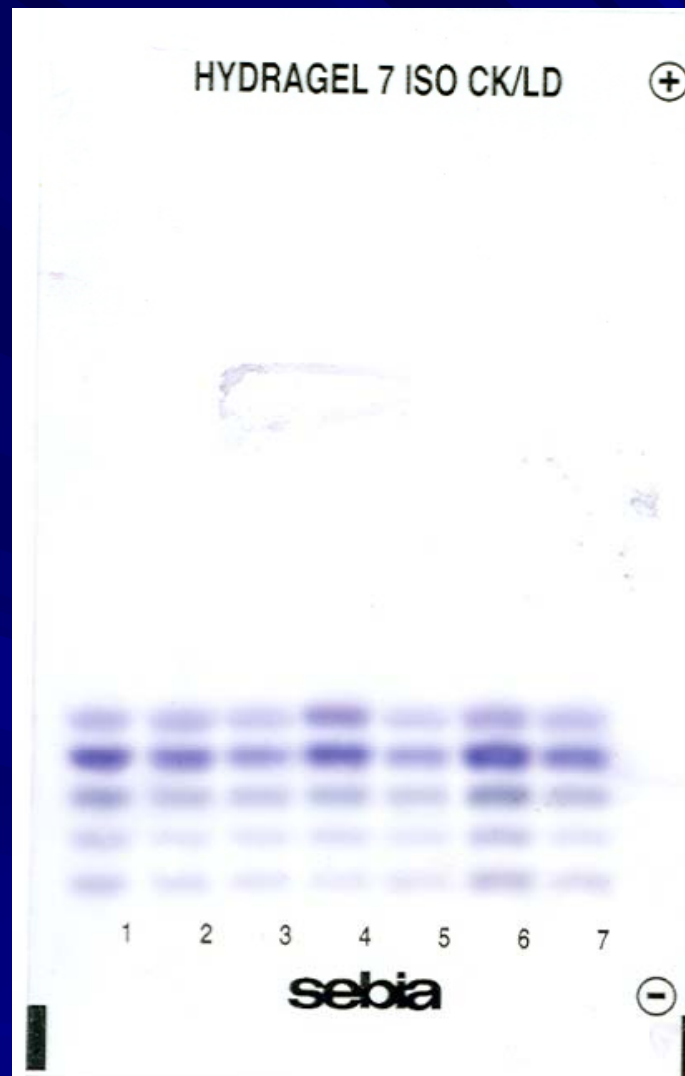
Photomicrograph No. 3.4 AGAROSE GEL SHOWING RAISED LD2 LEVELS AFTER ELECTROPHORESIS
